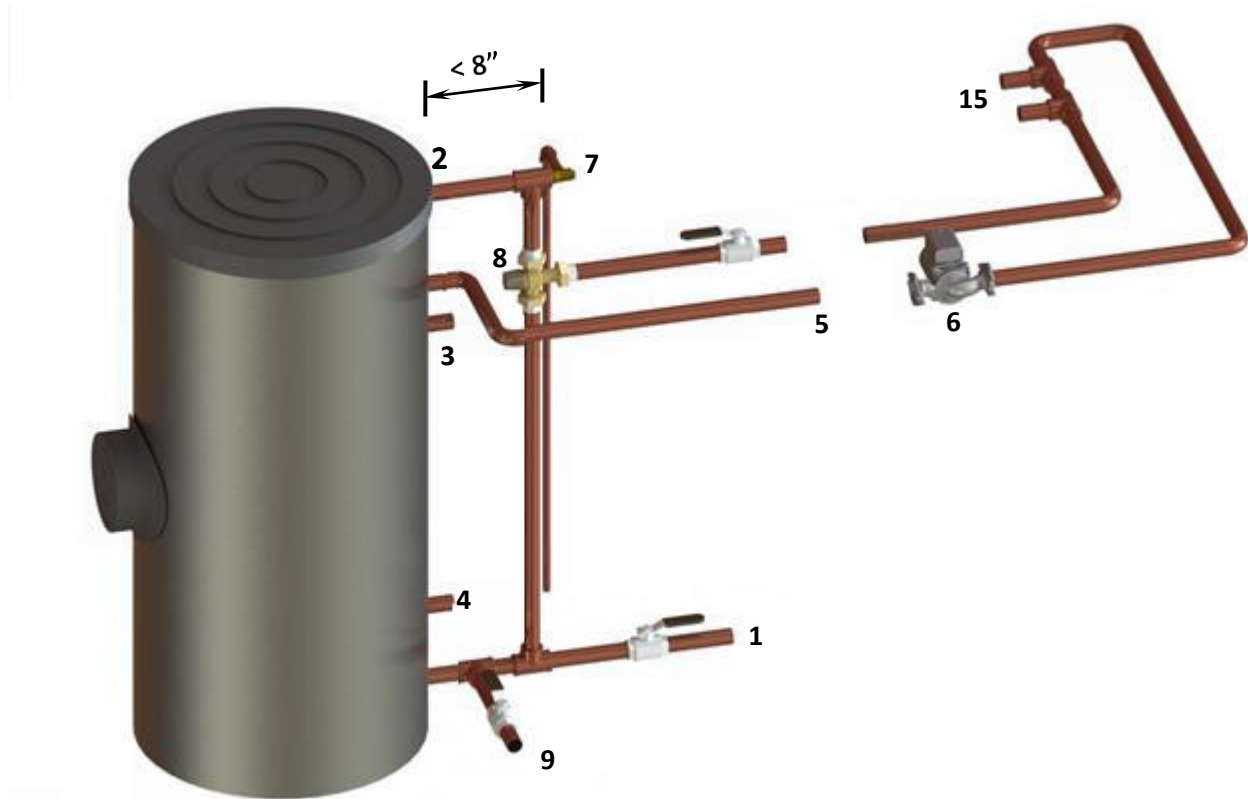
Figure 3. Tank Connections And DHW Service Recirculation Pump
